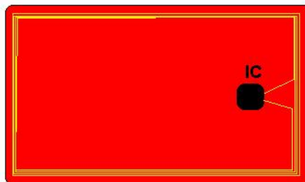
Figure 3. Internal view of a contactless smart card, with the antenna connected to the IC module.
